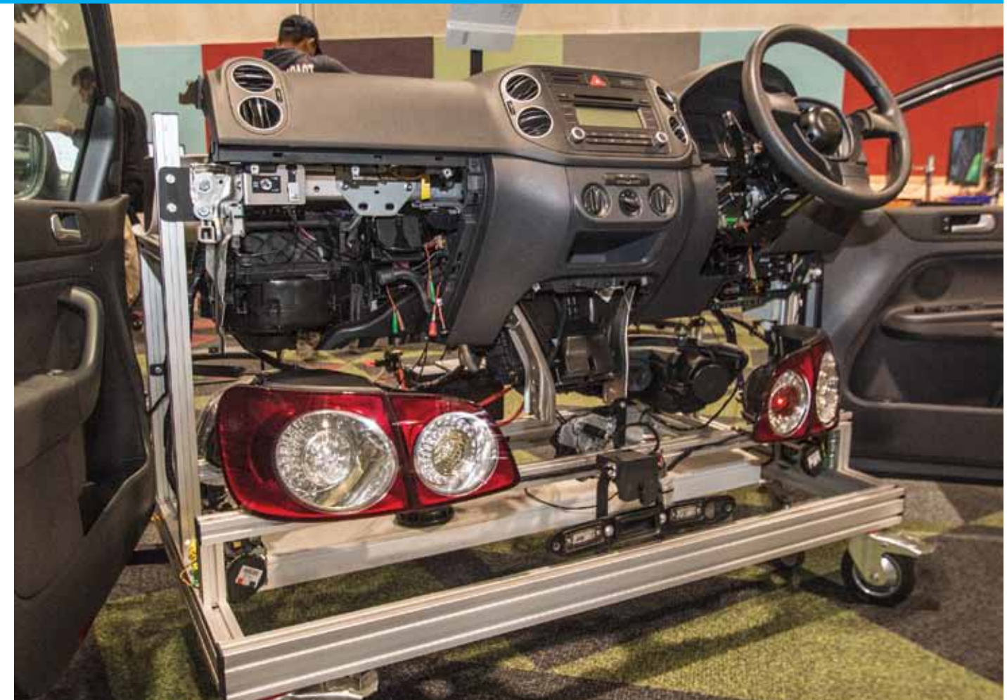
The front end of a VW Golf, which has been opened up to expose wiring and other componentry, allowing students to see and feel how it all fits together.
