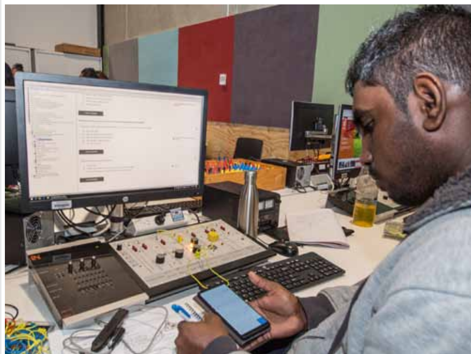
Sonali works with an automotive electrical fundamentals board.
